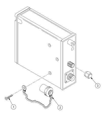
Figure 6: SD-44 replaceable parts
