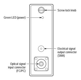
Figure 1: SD-44 front panel
