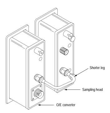
Figure 2: Using the rigid connector
