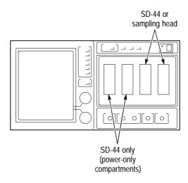
Figure 3: Front panel compartments in a CSA 803 Communications Signal Analyzer
